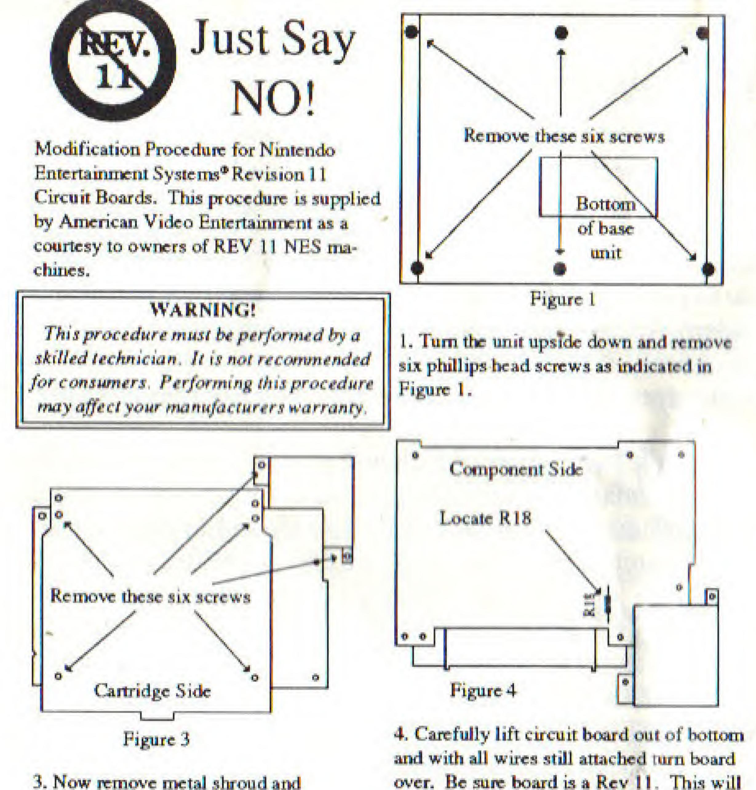
3. Now remove metal shroud and remove six phillips head screws as indicated in Figure 3.
